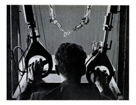
Dangerous object being handled: *M*[*G*]. Handles of the remote manipulator: forcing conditions.
