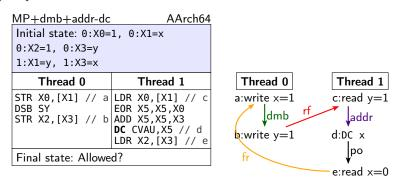
Same-Cache-Line Ordering ARMv8 has an architected cache line of minimum size. Accessible as the DMinLine and IMinLine bitfields of the CTR\_EL0 register, encoding the smallest cache-line size for the data and instruction caches, respectively.
